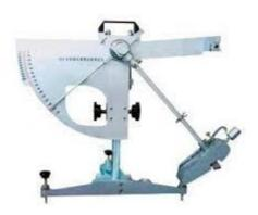
The British Pendulum Skid Tester gives a surface a P rating. The P rating can then be used to determine the correct Anti-Slip product to comply with AS 4586, and AS 4663, for a specified area. Although there is no direct correlation between a P rating and an R rating, compliance is demonstrated by achieving the value set out in the table below for either the wet pendulum test or the oil-wet inclining ramp test. It is not necessary to meet both criteria.
