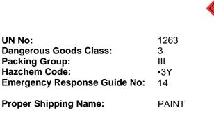
**Segregation Dangerous Goods:** Not to be loaded with explosives (Class 1), flammable gases (Class 2.1), if both are in bulk, toxic gases (Class 2.3), spontaneously combustible substances (Class 4.2), oxidising agents (Class 5.1), organic peroxides (Class 5.2), toxic substances (Class 6.1), infectious substances (Class 6.2) or radioactive substances (Class 7). Exemptions may apply.
