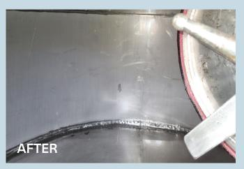
Images showing inside of tanks before and after using 0.52% w/v Vincirc Phosphate Free cleaning via a venturi system with 200L of cold water for 20 minutes.
